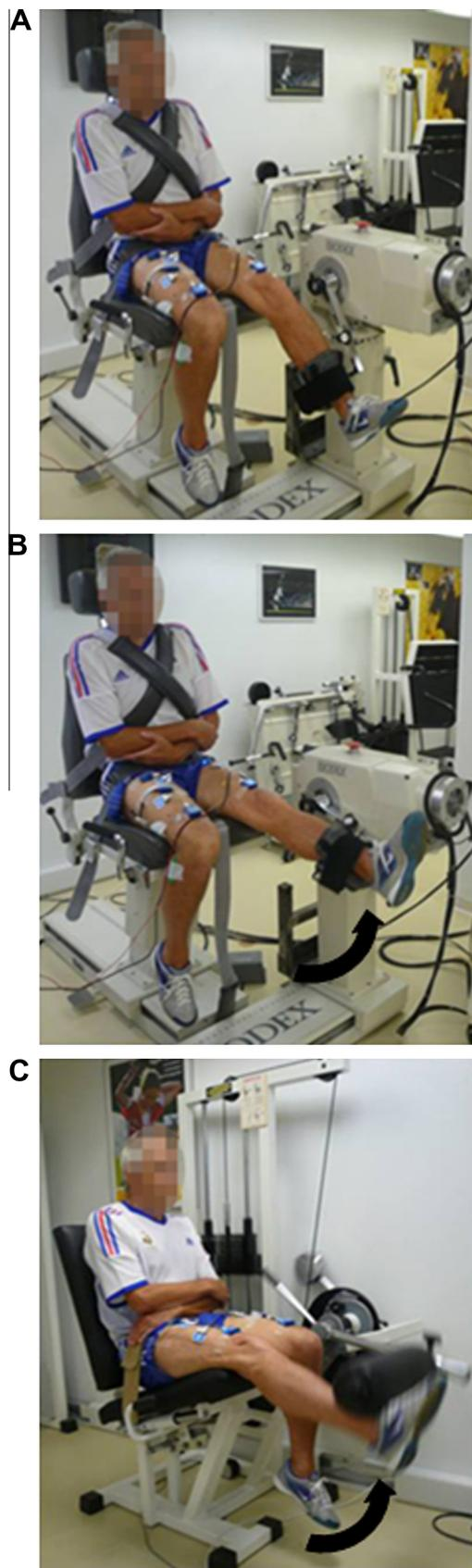
**Fig. 1.** Assessment of (A) isometric maximal voluntary contraction (MVC) torque, (B) isokinetic peak torque, and (C) isoinertial one-repetition maximum (1-RM) load.
